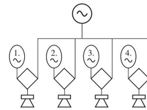
or the 4 sine-wave generators **unmodulated** are heard directly over 4 monitor loudspeakers, the volumes of which can be controlled by the players themselves.
